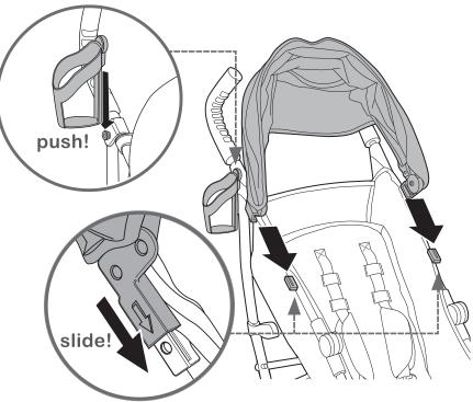
slide canopy onto frame mounts and attach velcro (both sides) 3
