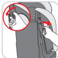
Release the safety catch (**SR**) of the safety bolt (**SB**) at the top of the back of the base unit (**BT**) and pull out the lower safety bolt (**SB**) sideways from the base holes.
