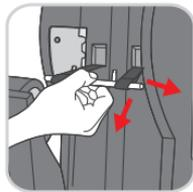
**Caution:** the safety bolt (SB) must lock the seat (ST) completely with the base (BT) again.
