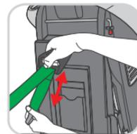
Now take the Top Tether (TT) and guide it under the head rest along to the appropriate Top Tether anchor point of the car.
