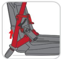
Tighten the three-point belt by pulling it closer to the three-point belt buckle (X). Now draw the diagonal belt (U) tautly upwards in the direction of the retraction mechanism. Fix the belt by closing and locking the belt clamp (GK). Now fold the seat (ST) back, secure the lower safety pin (SB) and the safety catch again.
