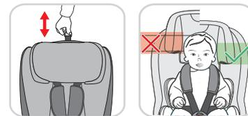
The headrest must be adjusted so that the distance between the shoulders of the child and the headrest does not exceed 3 cm (about 2 finger widths).
