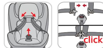
By pulling on the central adjusting belt (G5) make sure that the harness belts touch the child firmly and are not twisted.
