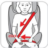
**IMPORTANT:** The diagonal belt should run centrally over the shoulder, the lap belt as low as possible over the groin.
