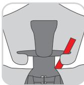
Let the shoulder strap of the vehicle run through the belt guide slot. The shoulder strap should run in the middle of the shoulder to ensure an optimal belt path.
