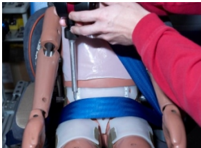
Right upper edge of lap belt at lateral location of ASIS
