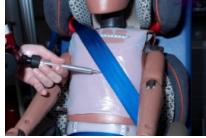
Lower edge of shoulder belt where it crosses the ATD centerline
