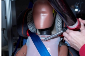
Upper edge of shoulder belt where it crosses the ATD centerline
