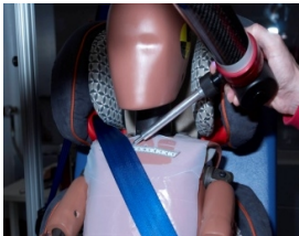
Inboard edge of shoulder belt where it crosses the ATD chest reference line
