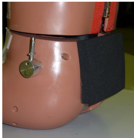
Figure 9 Pelvis Positioning Pad
