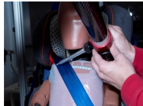
Outboard edge of shoulder belt where it crosses the ATD chest reference line
