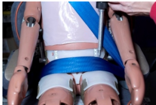
Left upper edge of lap belt at lateral location of ASIS
