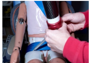
Right lower edge of lap belt at lateral location of ASIS
