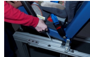
Test fixture reference point
