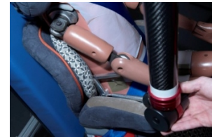
Right hip offset tool front
