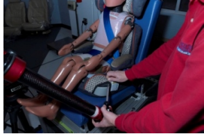
Front left reference point #1 on booster pan
