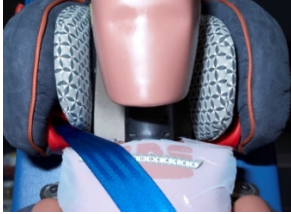
Shoulder belt hand measurement
