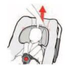
Release the switch and move the headrest until it reaches the nearest locking position, when you should hear a click. Check that it is locked by pulling the headrest.
