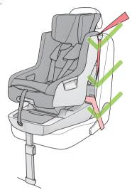
Check the correct position of the seat belts before each use. Please contact CONCORD directly if you have problems mounting the seat. The seat belts must run through the belt guides marked in red on the seat. The seat belt must not be laid out in any other way.
