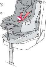
Place your child onto the seat as far back as possible. Bring together the shoulder/ lap harnesses and the central harness in front of the child and push the harness lock closed.
