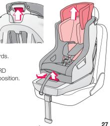
Open the harness lock of the 5-point harness system and fold the cover of the belt tensioner (06) upwards.
